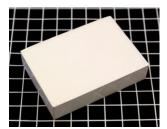
Airloy<sup>®</sup> X130 Series Composition: Polyurethane Features: Low cost, mid-range operating temperature, rigid-to-flexible Availability: Currently available on BuyAerogel.com
