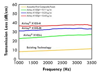
Thanks to their nanoporous structure Airloys provide superior sound transmission loss over traditional materials.
