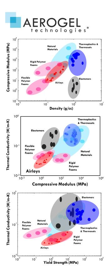
Airloys occupy a stiffness gap between foams and traditional plastics while still providing the durability and machinability expected of engineering materials and thermal conductivity and acoustic damping advantages.
