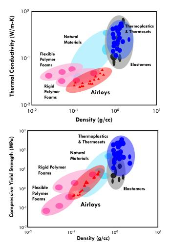
Airloys offer superior thermal insulating properties than traditional lightweight materials including polymer foams and wood while simultaneously offering excellent strength and stiffness.
