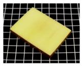
Airloy<sup>®</sup> X110 Series Composition: Polyimide Features: High operating temperature, non-flammability, low thermal conductivity, solvent resistance Availability: Currently available on BuyAerogel.com
